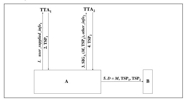
Figure 5: After Using a Scheme from 4.3, Entity A Requests a Second Timestamp
