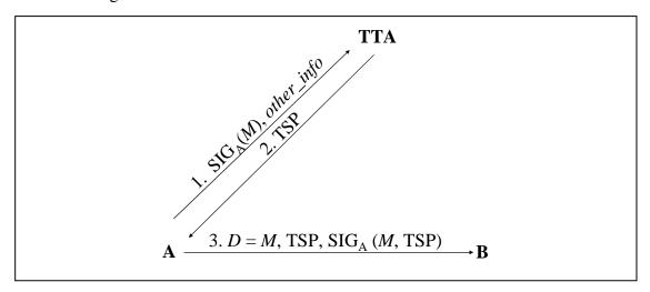
Figure 3: Entity A Provides a Signature to the TTA
